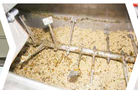
Food waste is mixed with microbes and broken down within 24 hours.
