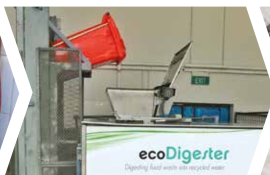
Food waste is loaded into the ecoDigester.
