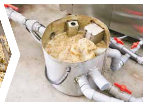
Non-potable water – the end product – is reused by the machine for self-cleaning.
